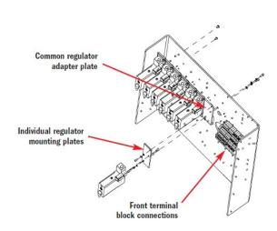
To make maintenance even easier, the Hard-Wired Zone Pressure Regulator Kit includes a front mount that simplifies the process of on-going maintenance. In addition, the original connection points have been retained for quick, routine maintenance checks.
