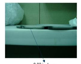
0.03 inch gap At 50K wafers processed, the Al Hub begins to show signs of warping; The Ceramic Hub maintains flatness integrity
