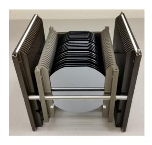
Equipment efficiency is critical to success in today's highly competitive chip manufacturing environment. CPS strives to provide enhancements that will improve tool availability. The 4" Nested Cassette provides for the processing of both 4" (100mm) and 6" (150mm) wafers with no changes to the equipment hardware.
