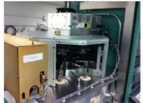
The upgraded Concept One RF Enclosure Assembly enhances the maintainability of the system and reduces the potential for safety incidents that can occur during routine maintenance.
