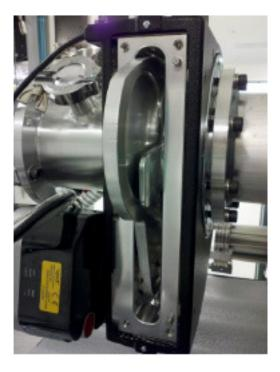
Concept Part Solutions is working to extend the lifetime of today's aging semiconductor manufacturing equipment. Component obsolescence and reliability are driving suppliers to provide innovative improvement upgrades to meet these demands. The C1 Heated Pendulum Valve is a system enhancement that will provide greater reliability and extendibility for the Concept One System platform.
