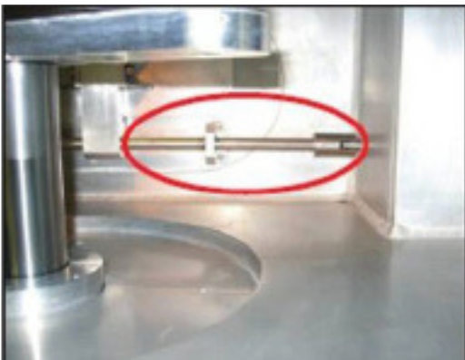
Current Load Lock Door with 2-piece shaft causes unwanted rubbing and particle shed
